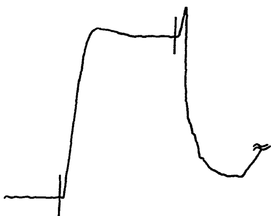
Fig. 3: Heat flow after addition of \text{Cr}^{++} using a flow microcalorimeter equipped with a flow through cell.
